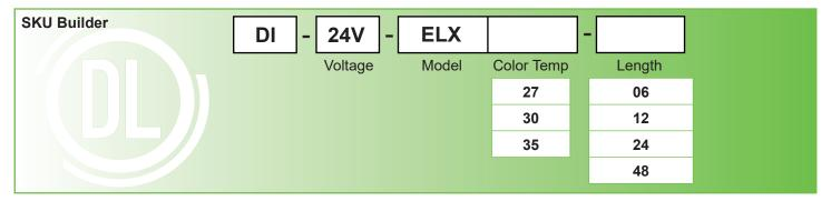
Example: DI-24V-ELX-30-24 = Diode, 24 Volt, ETERNALUX™ LED Light Bar, 3,000° CCT, 24.13 inch length
